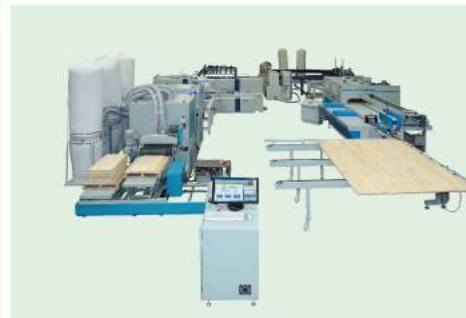
| Automatic Wood Boarding Line
